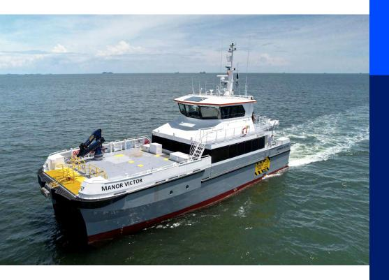
Manor Victor is a multi-purpose offshore crew transfer vessel designed to transport personnel and equipment to and from offshore wind farms.
