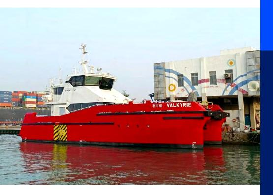
Valkyrie is a multi-purpose offshore crew transfer vessel designed to transport personnel and equipment to and from offshore wind farms.
