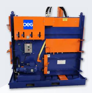
OEG's **ENVIRO**PAK 4000CB is designed for simple, safe, and reliable operation. The double chamber design allows for in bag compaction on one side while a cardboard baler on the other. Featuring a hydraulic operated roll back top for easy loading and unloading, the CB-series compactors efficiently manage all types of non-hazardous waste.
