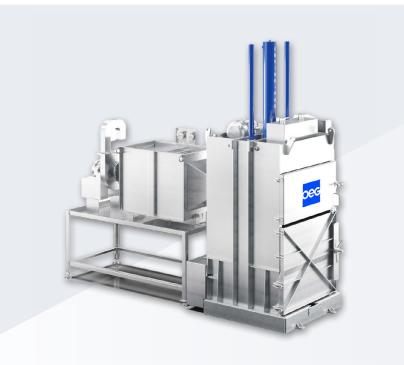
OEG's **ENVIRO**PAK 4000HM waste compactors compact hazardous waste inside UN/DOT approved 1 cubic yard corrugated disposable shipping containers with up to 60,000 pounds of compaction force. Compaction force is transferred directly to the compactor walls, eliminating distortion of the container.
