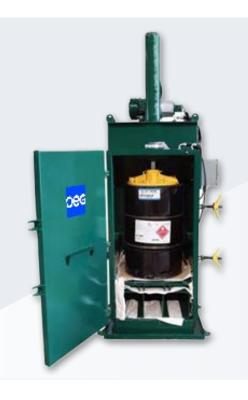
OEG's **ENVIRO**PAK drum crushers compact waste into 55/85 gallon drums before crushing the waste further. The Drum Crushers can crush 55 gallon drums to 4" and reduce disposal costs of hazardous waste by compacting into UN/DOT approved drums. All units meet and exceed international MARPOL 73/78 Annex V and utilise UL listed components.
