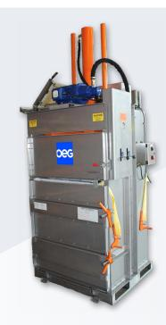
OEG's patented **ENVIRO**PAK stainless steel vertical balers are constructed from 316 stainless steel and bale paper, plastic bottles, and cardboard. Component parts are sand blasted and painted for corrosion protection. All balers meet and exceed international MARPOL 73/78 Annex V and use UL listed components.
