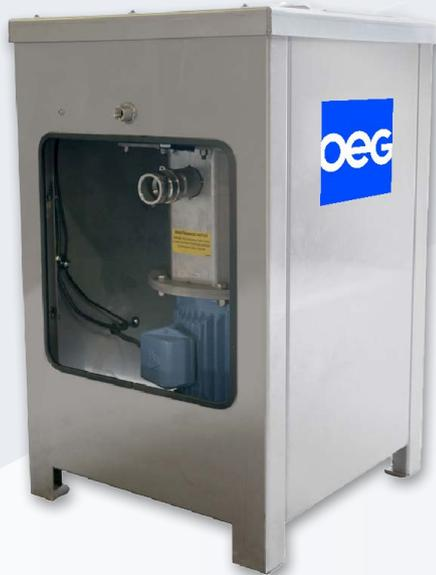
OEG's **ENVIROPAK** Tuff gut II food grinders are designed for galley installation, but are suitable to withstand outdoor elements, built with an all stainless-steel structure and grinding components. The Tuff gut II is delivered ready to connect to the water supply, discharge and power supply for easy setup. All units meet and exceed international MARPOL 73/78 Annex V and IP55 protection class.
